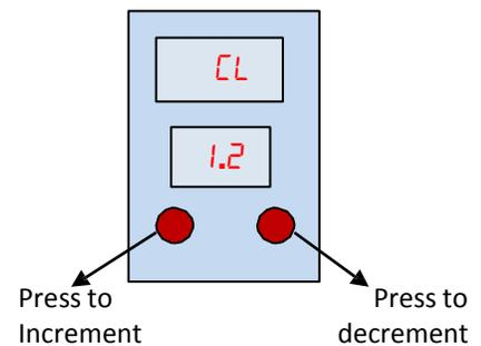
Press both buttons together to save the changes. The unit returns to its normal display after saving the new current limit.
