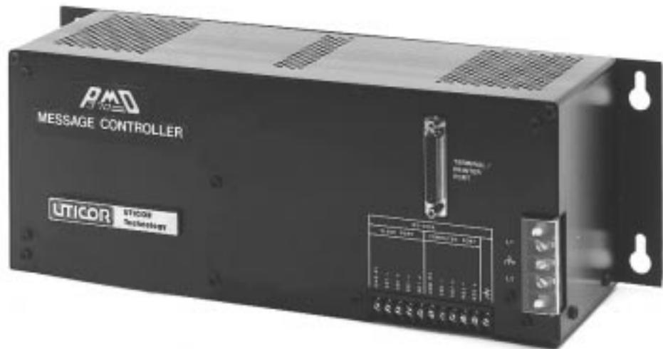
The PMD 300MC Series Programmable Message Controller is essentially a PMD 300MC Series Master Message Display without the built-in vacuum fluorescent display. It allows you to store message programs, log messages, operate slave displays, communicate via computer interface, and all other PMD 300MC operating features except that it requires a slave display to view its messages.
